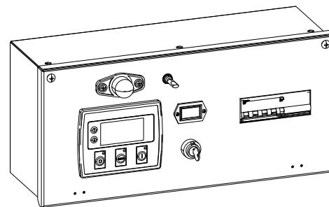
PLC-920 is an advanced control module based on microprocessor designed to control the engine via push buttons on the front panel. The module is used to start and stop the engine and indicate fault conditions, automatically shutting down the engine and giving a true first up fault condition of an engine failure.
